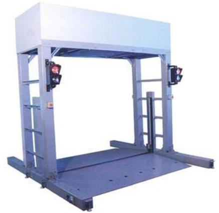
Conventional vehicle scanners require the driver and passengers to leave the vehicle prior to the scanning taking place to prevent harmful radiation exposure, this obviously slows the through put of vehicles to approximately 30 per hour and there is still a potential risk that the occupants may be carrying explosives.
